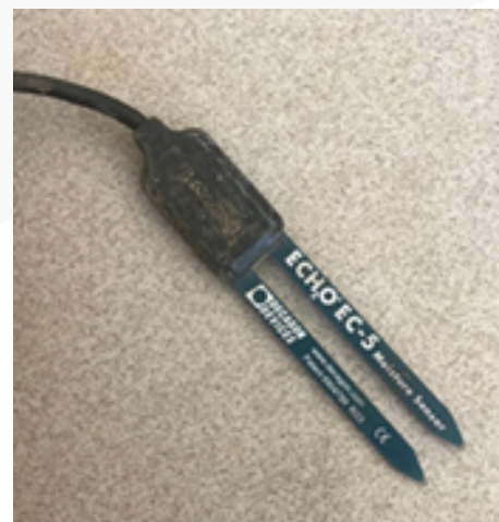
Figure 6. Meter© EC-5® Capacitance Sensor.
