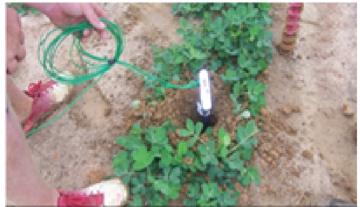
Figure 4. WaterMark soil water tension sensors installed in a probe
