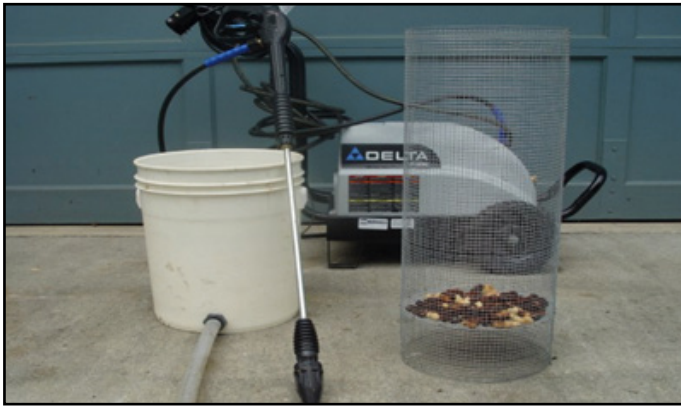
Figure 3. Pressure washer with orbital nozzle to blast on outer layer (exocarp) of hull. Source: CAES. Miscellaneous Publication No. ENG 03-004.
