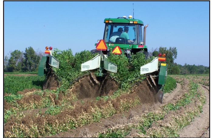
Figure 1. Planting peanuts using and RTK-based auto-steer system (left) and inverting peanuts using and RTK-based auto-steer system (right).
