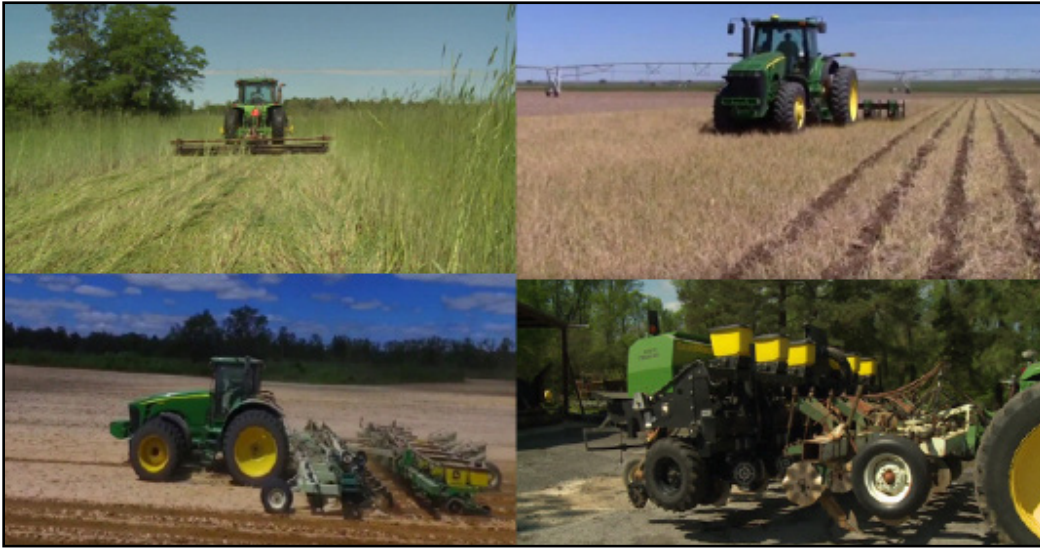
Examples of reduced tillage practices. Top:rolling of cover crop before tillage operation (left) and ripping into covercrop residue before planting (right). Bottom: two pictures of a 1 trip rip and plant combination used in reduced tillage. Images courtesy of Kris Balkcom, Auburn University
